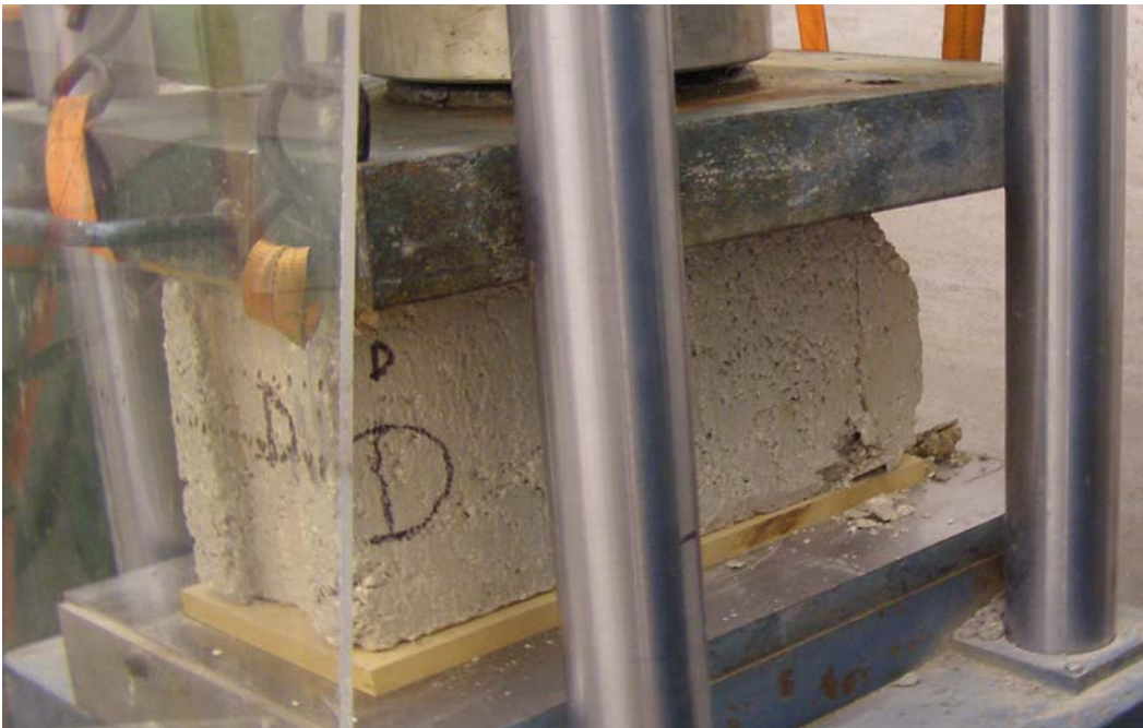
Block D at failure (note vertical crack at the right end of the block and crushing at the base)
