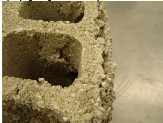
Delamination of the face shell and crushing of the web between two hollow cores
