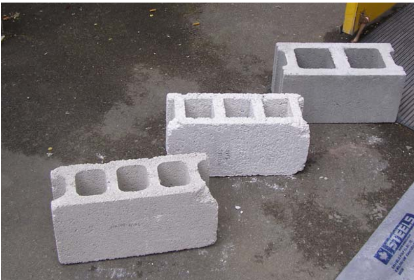
Haiti blocks C and D (6 inch thick), and a Canadian block (8 inch thick) (from left to right)
