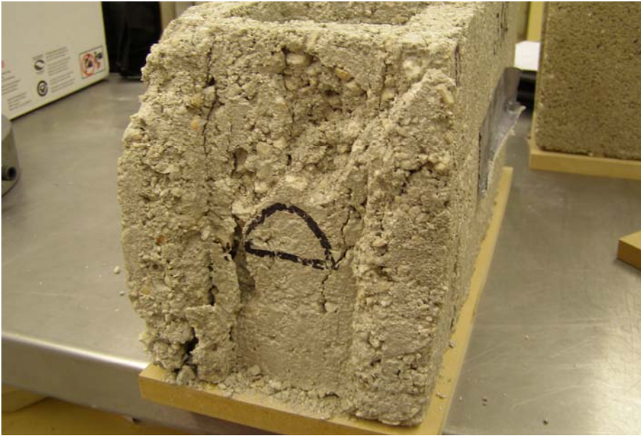
Damage at the rear side of the block, showing cracking in the web
