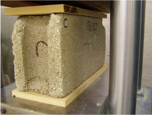
Block C before the testing (note fibreboard capping)
