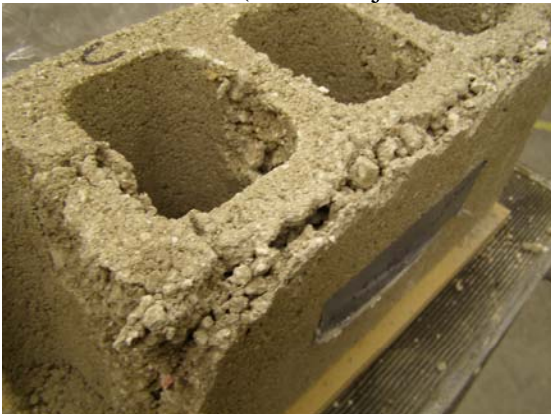
Delamination of the face shell and crushing of the web between two hollow cores
