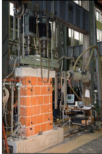
Figure 11. Test set-up and instrumentation of walls for cyclic lateral resistance tests
