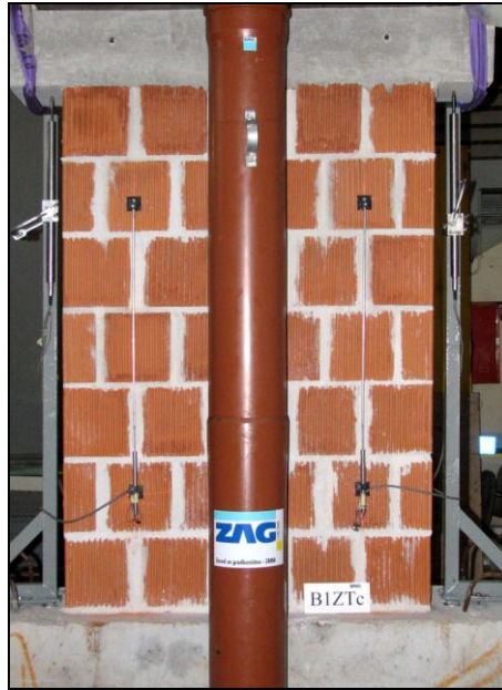
Figure 8. Disposition and instrumentation of walls during compression tests
