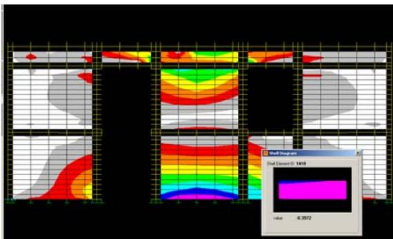
Figure 6a. Envelope values of M22 bending moment.
