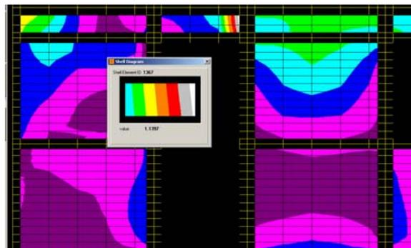
Figure 6b. Envelope values of M11 bending moment.
