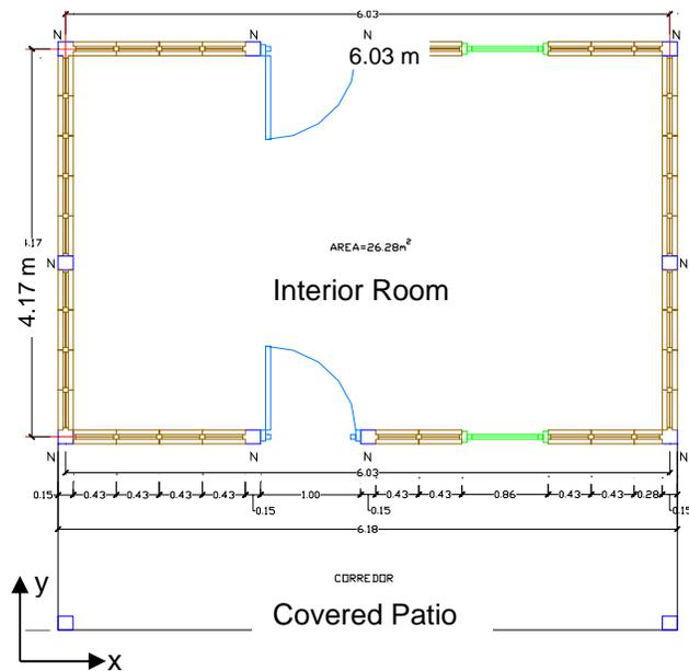
Figure 4. Plan used in analyses of mixto house.
