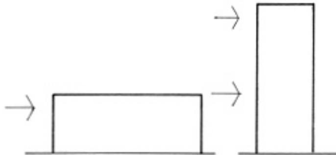
Figure 4. Overturning effects of horizontal loads.
