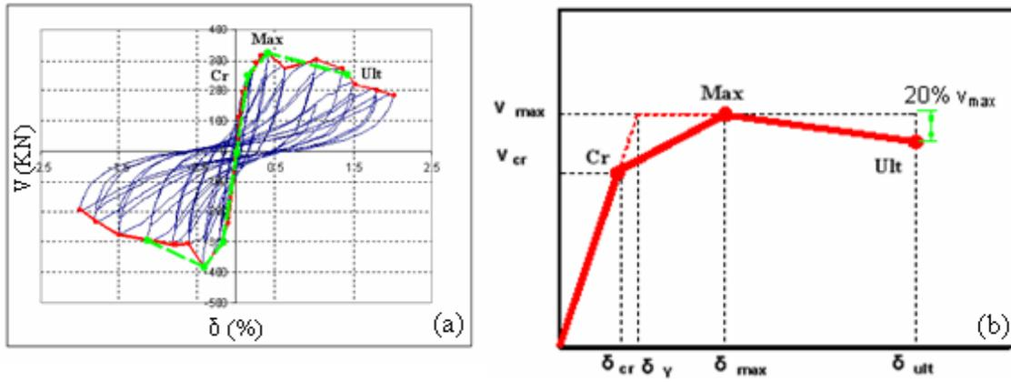
Figure 3: (a) Example of determination of model parameters on the basis of the recorded response (Specimen M-147, Ishibashi et al., 1992), (b) Backbone model of the current study
