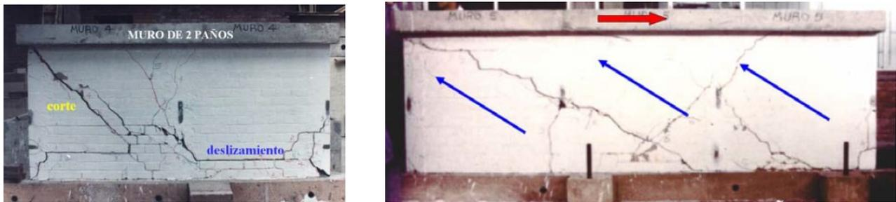
Fig. 5 – Effect of the number of wall panels in a 1/2 scale masonry model [6].
