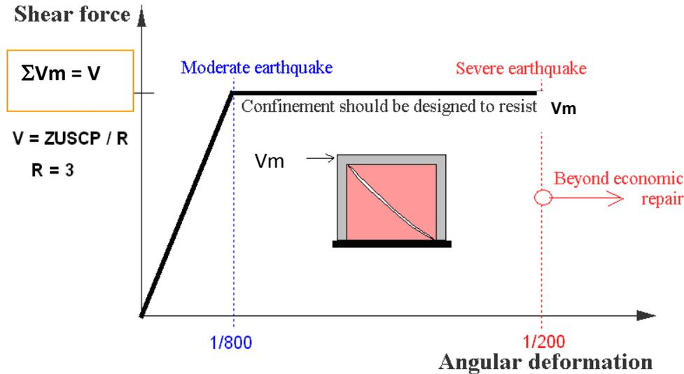
Fig. 7 – Objectives of the design procedure [11, 12].
