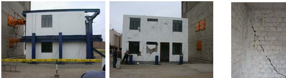
Fig. 9 – Test on a full scale two-story masonry house at UNI-CISMID.
