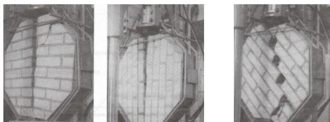
Fig. 2 – Octagonal masonry specimens tested by Gallegos [8].
