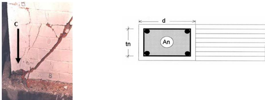
Fig. 8 – Vertical confinement (tie-column) design forces and cross section [12].
