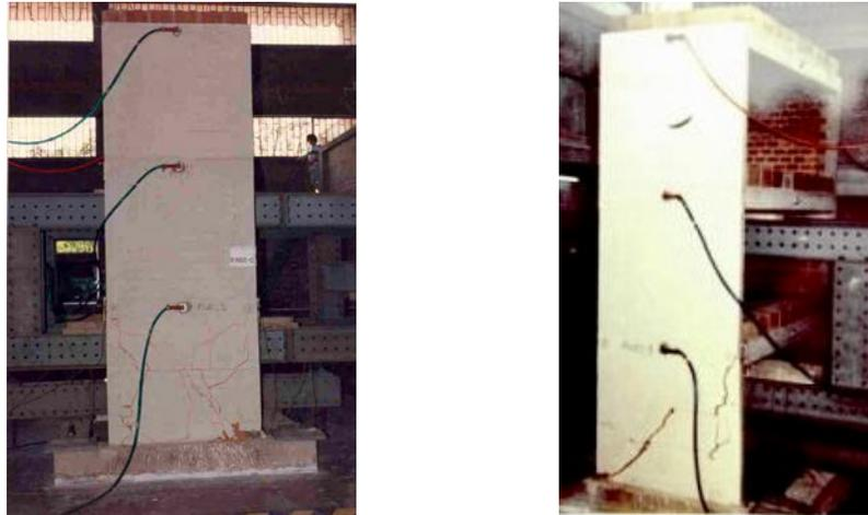
Fig. 4 – Shaking table test on 3-D masonry model [10].
