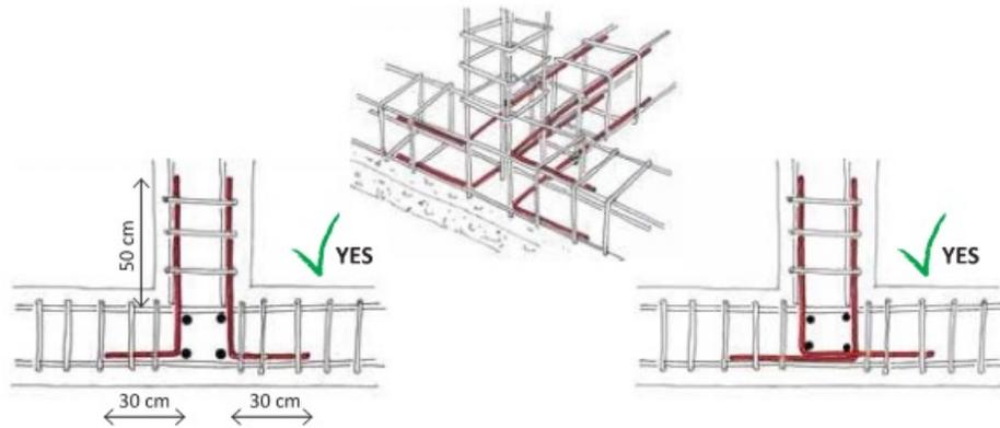
Fig. 3 – Recommended beam to beam connections [6]
