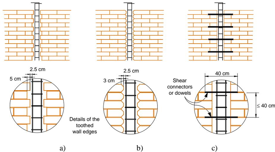
Fig. 2 – Tothing in confined masonry walls: a) machine-made hollow units, b) hand-made solid units, and c) provision of horizontal reinforcement when tothing is not possible [3]
