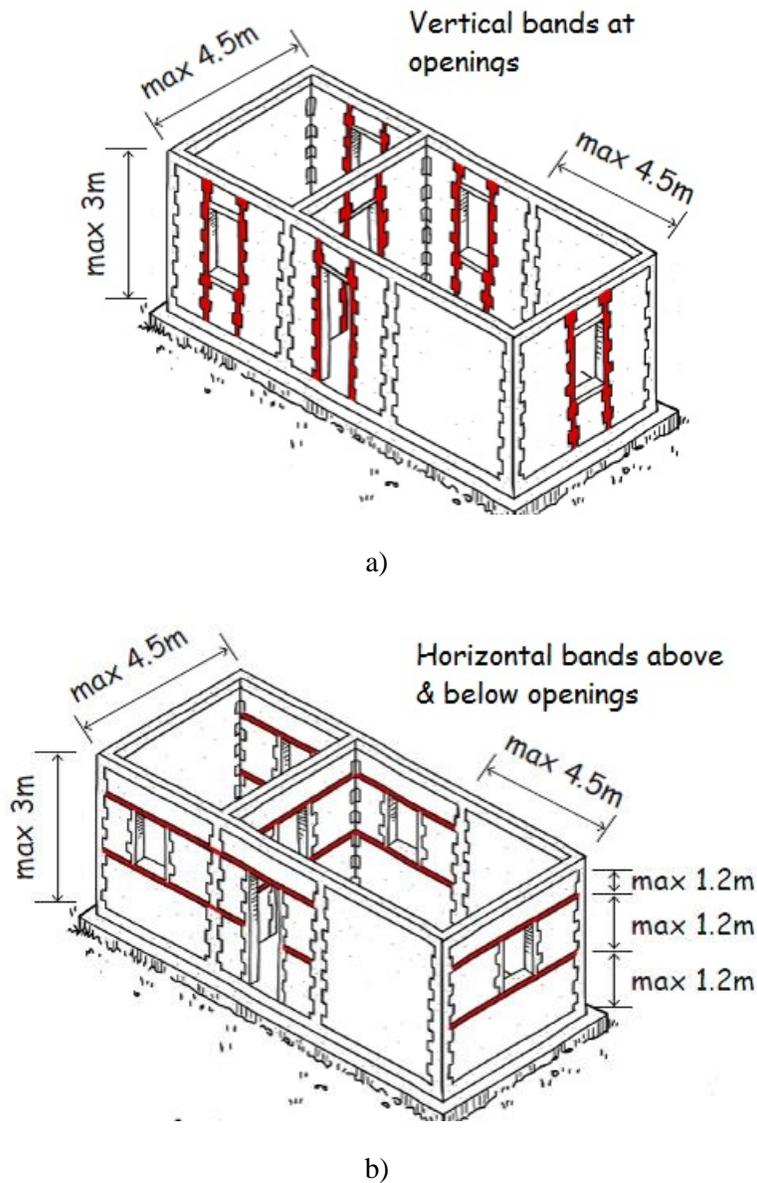
Fig. 5 – Reinforcement in confined masonry buildings: a) vertical RC ties, and b) horizontal RC bands [12].
