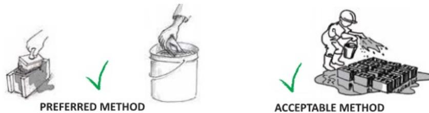
Fig. 4 - Wetting the masonry units prior to installation [6]
