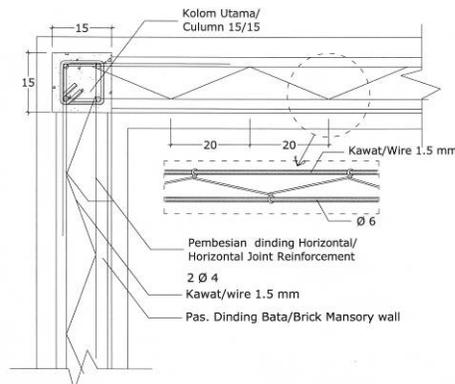
Fig. 4 - Horizontal Bed Joint Reinforcement
