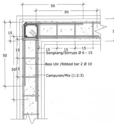
Fig. 8 - Beam/Column Intersection
