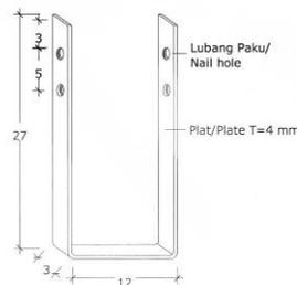
Fig. 6 - U-shaped plates used at trusses
