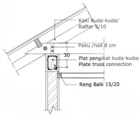
Fig. 5 - Truss to Ring Beam Connection
